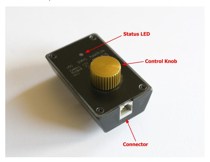
Turning the knob clockwise normally produces clockwise motion of the focuser and counterclockwise produces counterclockwise motion. The relationship between knob direction and "in/out" motion depends on the mechanical design of the telescope focuser, but it can be changed in the setup of the focus controller. Refer to section 5.2.4.2 for details.
