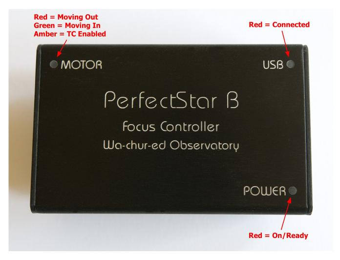
The LEDs are fairly small and dim, so as not to disturb night vision adaptation. The power indicator should light up in red when power is supplied. It does not turn on until the controller has completed its initialization. Note that this LED does not necessarily mean that the source voltage is adequate to power the motor.
